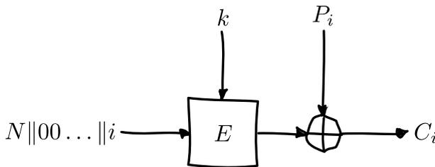
Figure 7.4: *CTR mode*: a single *nonce*  $N$  with a zero-padded counter  $i$  is encrypted by the block cipher to produce a keystream block; this block is XORed with the plaintext block  $P_i$  to produce the ciphertext block  $C_i$ .
