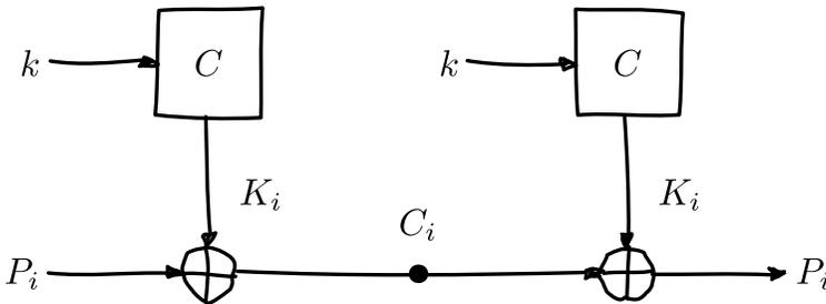
Figure 7.3: A synchronous *stream cipher* scheme. Note similarity to the one-time pad scheme. The critical difference is that while the one-time pad  $k_i$  is truly random, the keystream  $K_i$  is only pseudorandom.
